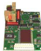
Fig. 9 TCM2-20 biaxial inclinometer and a triaxial magnetometer compass module
