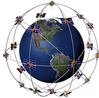
Fig. 11 Diagrammatic representation of the 24 satellites of the Global Positioning System
