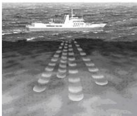
Fig. 5 Diagram of transmission principle of an Acoustic Doppler Current Profiler, mounted onboard a ship, showing the 4 directions of the 4 beams
